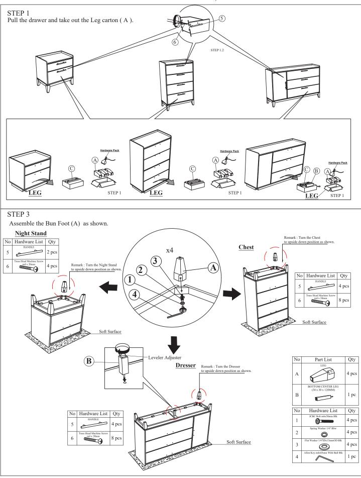
NOTE : MUST TIGHTEN SCREWS PERIODCALLY WITH USE SCREW WILL BECOME LOOSE CHECK TIGHTNESS OF ALL SCREW EVERY 6-8 WEEKS.
